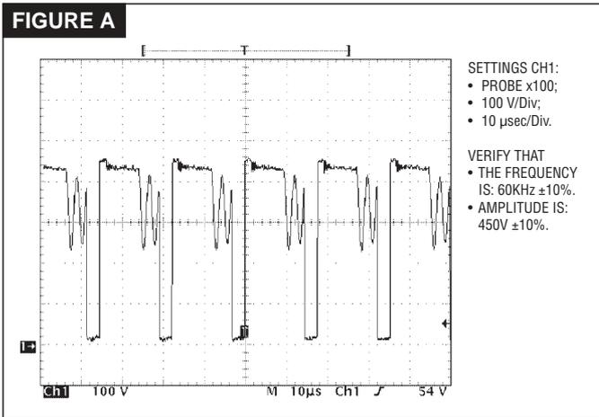
**N.B.** if no signal is present, it may be necessary to replace the integrated circuit U2 (**fig. 3**).
